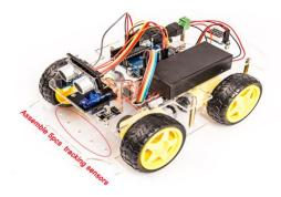
C. Make sure every sensor head is over the gap at the front of the lower chassis so that the sensor will be able to detect a black line on a white background.
