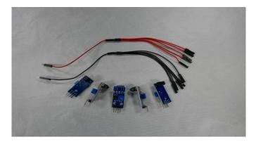
B. Attach the 5 tracking sensor modules into the empty holes at the front of the lower chassis.
